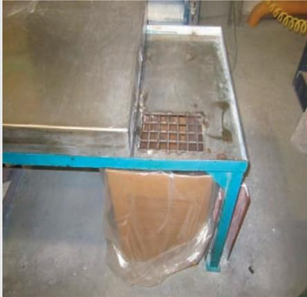
Improve weighing provisions by collecting spilled materials in drums
