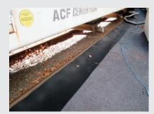
Small quantities of pellets can be lost during unloading at a rail siding. The track bed with stones hinders proper cleaning, so after the original track bed had been cleaned, a small blacktop culvert was added along the unloading area to simplify the cleaning process for this area.
